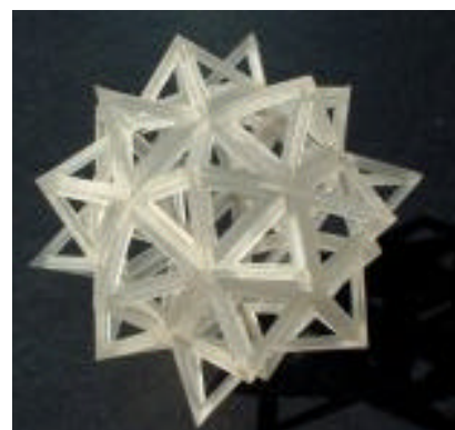
A plastic stereolithography model, 8 centimeters in diameter, of an "elevated rhombicuboctahedron," originally depicted by Leonardo da Vinci.
